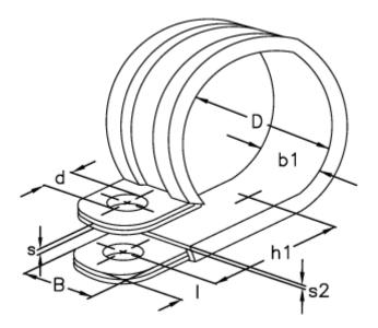
$\begin{array}{lll} \text{b1} & = 18.5 \\ \text{d} & = 6.4 \\ \text{Diameter D} = 13 \\ \text{h1} & = 17.7 \\ \text{I} & = 6.0 \\ \text{s} & = 0.60 \\ \text{s2} & = 1.5 \\ \text{Width B} & = 15 \\ \end{array}$
